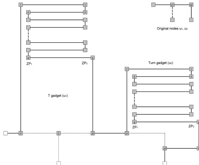
Figure 4: A T gadget and a Turn gadget that correspond to the node  $u_1, u_2$  of the portion of the grid graph shown in the upper right corner. The bold polyline shows a valid traversal that enters the Zigzag points of both gadgets.
