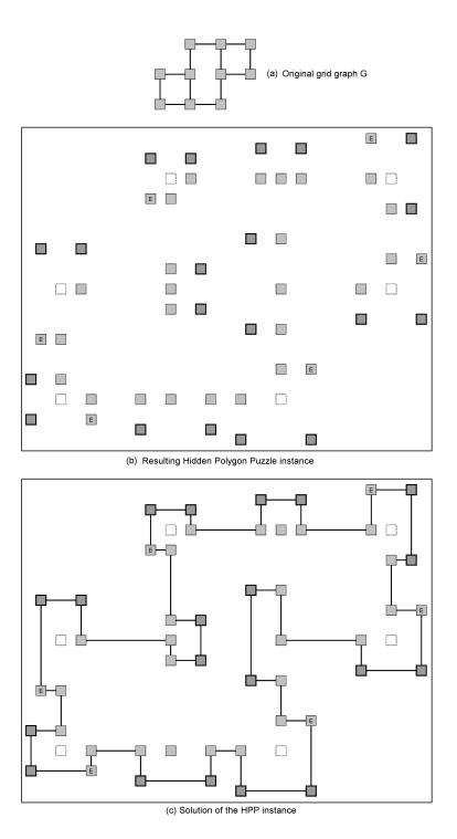
Figure 5: a) A grid graph G with n = 10 nodes and b) the corresponding HPP instance with k = 220. The Zigzag points are collapsed to make the drawing more readable; each bold box contains  $\tilde{h}$  Zigzag points. The bottom drawing c) shows a simple rectilinear polygon with 230 > k vertices that is a valid solution and that corresponds to an Hamiltonian cycle on the original grid graph.
